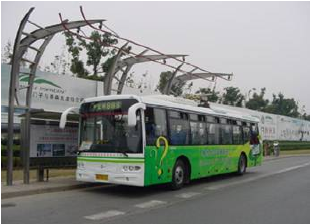
Photo showing Sinautec Ultracap Bus in operation in Shanghai
